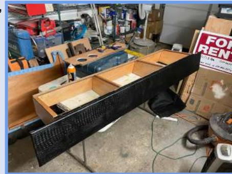
base. Then using the original wood as a template I cut out new pieces from the marine plywood I bought. The West Systems epoxy is nice because they have pump handles that screw into the resin and catalyst and each pump is metered appropriately. All you have to do is pump as much resin into a cup as you need and match it with equal pumps from the hardener. Once these
