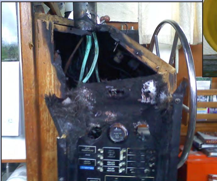
in that you were sending all of the shore current through an internal shunt which over the years would cause heat inside the gauge. Having a separate inductive coil shunt that fits around the incoming wire is much safer because there is no coil that the power feeds through.
