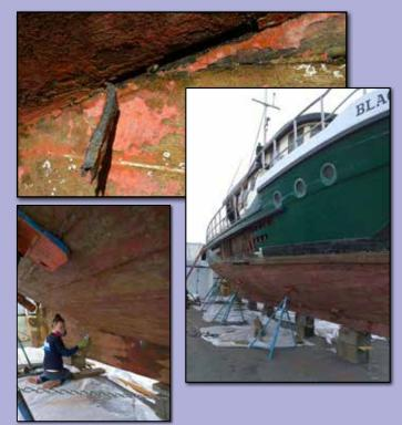
While Alan was working on the ever growing hole in the side of the boat, Alan's son Aaron, my friend Michelle and I worked on scraping the bottom, cleaning up smaller bits of rot and patching gouges. This continued well after Alan was done. Turns out there is a lot of bottom on a 50-foot displacement hull. It was hard not to get carried away and fair everything to perfection. But as Alan kept reminding me it is not a Chris Craft, it is an old work boat.
