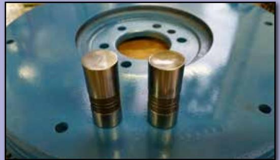
Talking with Delta Camshaft in Tacoma, Scott asked if I had done a lot of idling, well yes I did. He said this was a problem with this type of engine. He helped me with a new cam and lifters. On the lifters he showed me where they put a thin flat spot along the side with a stop to pull oil down to the cam lobe to prevent the lifters from dishing in. Hope this works.
